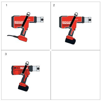
Position of the securing strap at Ridgid press machines:
