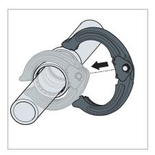
Open the press ring and place it around the respective pressing point of the fitting.
