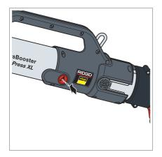
Keep the button for manual unlocking pressed until the piston has fully retracted and the hinged adapter jaw is no longer stress loaded.
