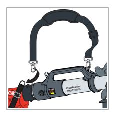
Use clasps to fasten the strap ends to the PressBooster and the press machine as shown.
