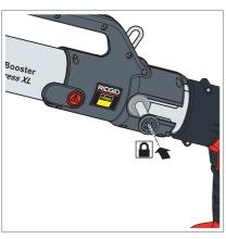
Slide the retaining bolt of the press machine in as far as it will go.
